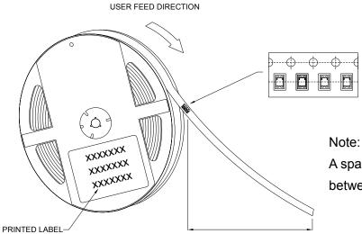
A spacing of approximately 160mm between the front edge of tape
